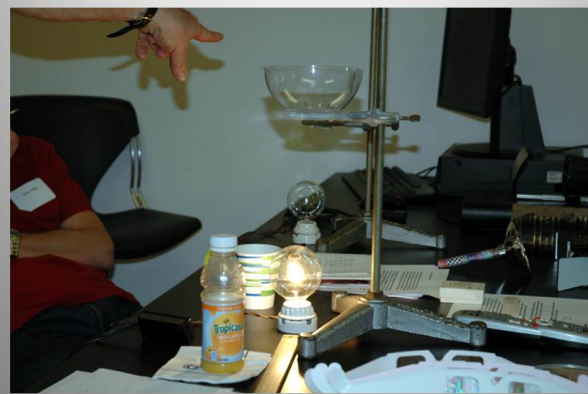
A "water lens" forms an image of the bulb on the ceiling
